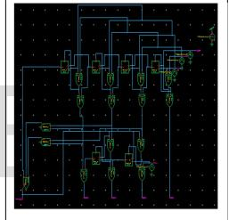
Fig.2 BCD ADDER USING XOR-MUX
